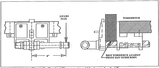
Figure 2: Product Placement and Maximum Applied Torque
